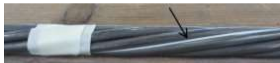
Figure 4. Pre-stressed steel strand instrumented with a GFRP optical fibre with 19 FBG sensors.
