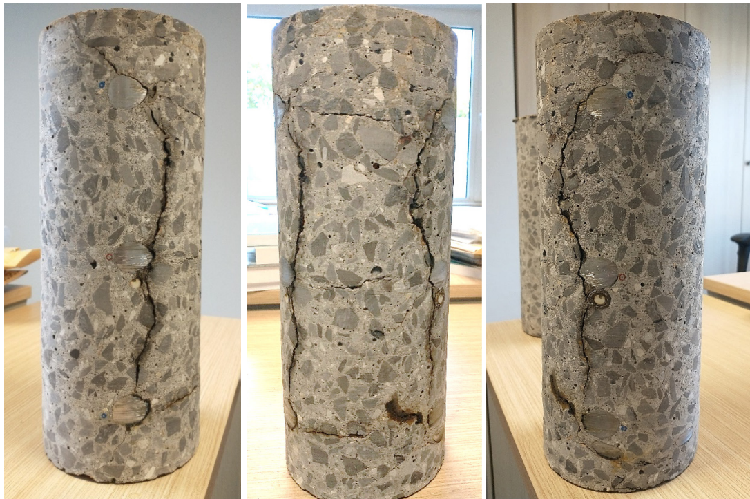
Figure 76. Pictures of a horizontal core drilling executed in beam B02 at the level of one of the point loads at the height of the lower longitudinal rebars.
