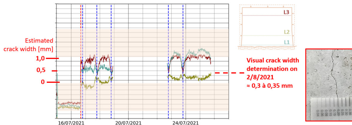
Figure 71. Estimation of the crack width of crack 2 by means of the Solifos V9 monitoring data (BOFDA DAQ unit), based on the validation experiments executed on notched beams.
