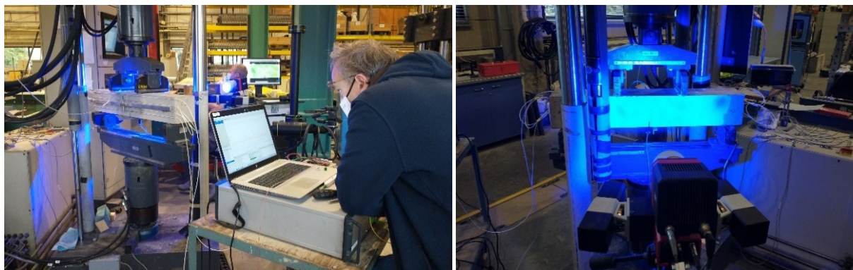
Figure 66. The experimental setup for the crack formation detection.
