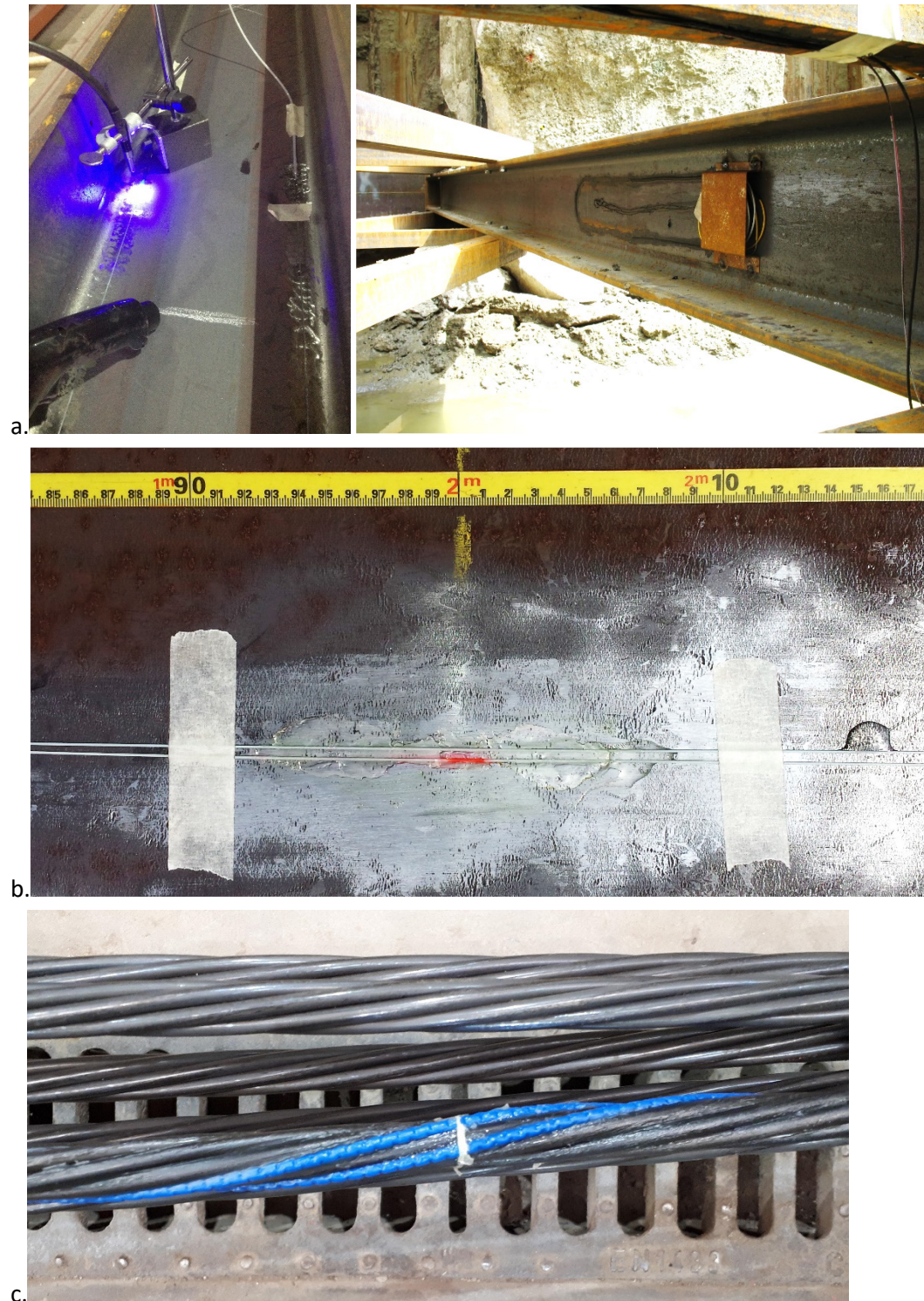
Figure 50. Examples of chemical fixation of sensing fibers. In the example of picture (a), the fiber will be glued inside the groove, which offers an additional protection.
