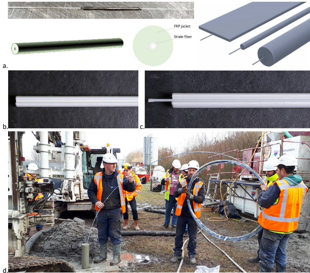
Figure 43. (a) The Fiber Sensing Rod as manufactured by Com&Sens with embedded FBG sensors. The fiber is coated with PET or glass fiber reinforced plastic (mono-acrylate resin). Diameters from 0.8 to 2.2 mm can be created. (b) GFRP rod (6 mm diameter) with a longitudinal notch (2mm deep and wide) as applied at the Buildwise. (c) The GFRP rod (6 mm diameter) with a GFRP coated fiber (1 mm diameter) in the longitudinal notch. (d) In field installation of the GFRP rod with integrated FBG sensors in a 70 m deep micropile.
