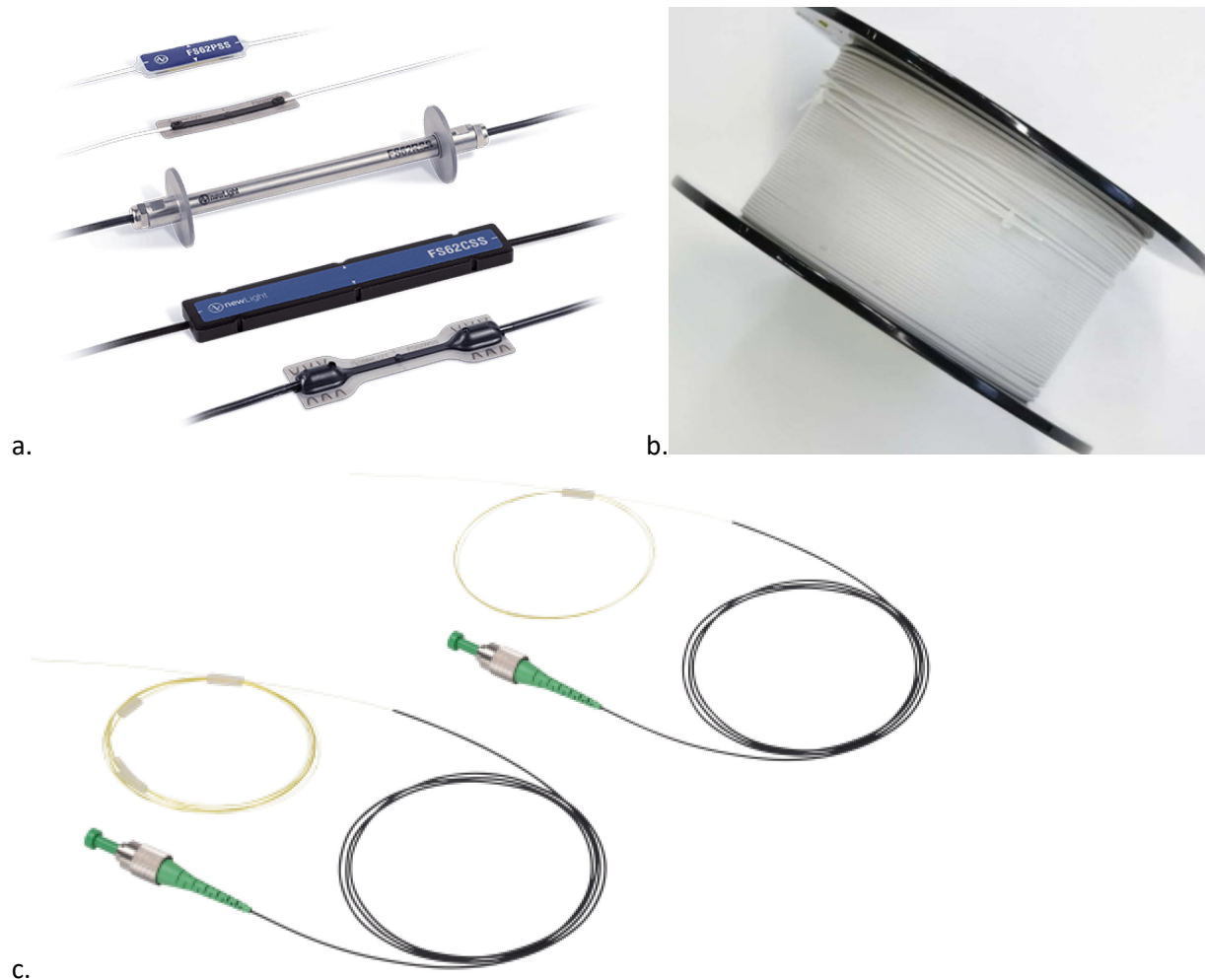
Figure 35. FBG strain sensors. (a) Surface mountable (by welding, gluing, ...) and embeddable strain sensors (HBK FiberSensing). (b) 2mm GFRP coated FBG array (FBGS). (c) Polyimide coated FBG sensors (Luna).
