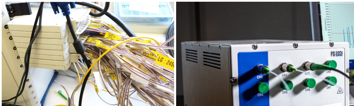
Figure 2. (left) 96 temperature sensors connected to a data acquisition (DAQ) system. (right) 3 sensor arrays connected to a FBG interrogator. Each array or each single cable could contain up to 30 sensors.
