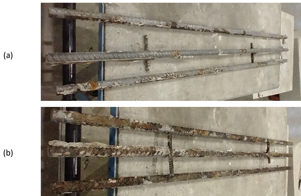
Figure 32. Pictures of the bottom rebars after the accelerated corrosion experiment: (a) top view and (b) bottom view.
