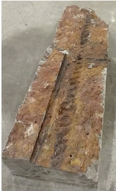
Figure 34. Picture of the crack surface of one of the splitting cracks of beam B02 after the accelerated corrosion experiment.
