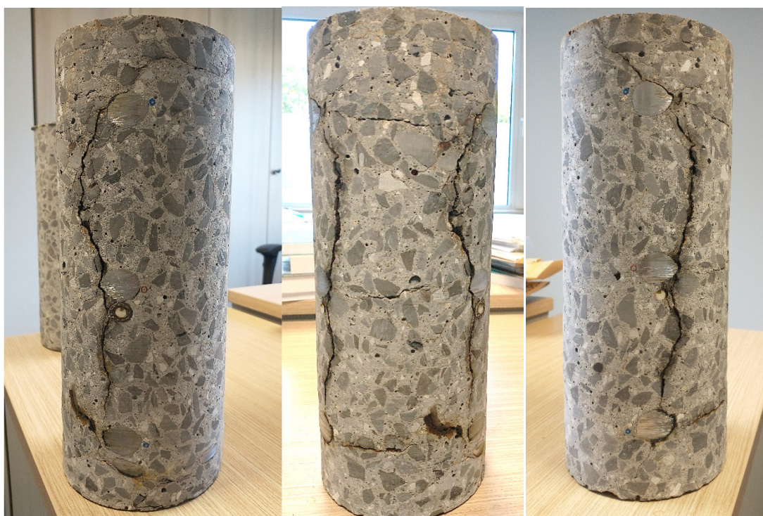
Figure 33. Pictures of a core drilling executed in beam B02 at the level of one of the point loads at the height of the lower longitudinal rebars.
